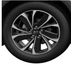
19" alloy wheels (machined spokes with polished finish and dark painted pockets)
