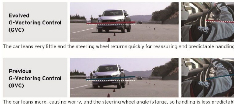
The car leans more, causing worry, and the steering wheel angle is large, so handling is less predictable
