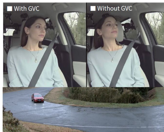
* In-house passenger seat comparison of left-hand turn at 30 km/h (lateral acceleration of 0.4 G)
